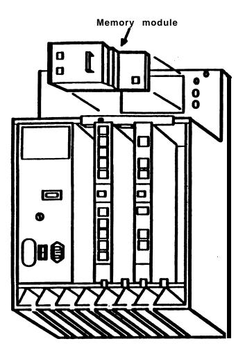
Figure 3 Inserting and Removing the Memory Module
